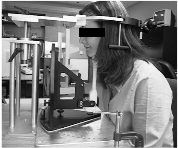
Figure 2. Head anchor and transducer holder for sonographic examinations.
